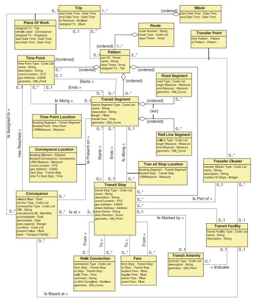
**Figure 2** Top-level view of a land use-based transportation hub siting database schema. The full schema has over two hundred feature classes
